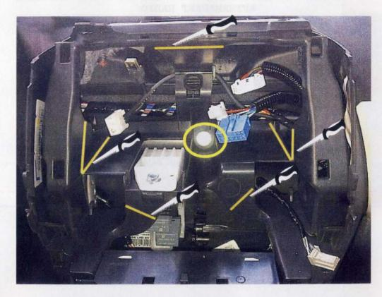
CUT OEM DASHBOARD IN THE POSITIONS SHOWN IN THE PICTURE, UNSCREW THE CENTRAL SCREW POSITIONED ON THE BOTTOM, AND REMOVE THIS PART TO ALLOW THE FIXING OF THE AFTERMARKET RADIO.
