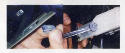
FASTEN THE PLASTIC HOLDER ON THE METAL PLATE SUPPLIED USING THE OEM SCREW AND CLIP
