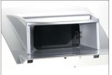
12. Connect all required circuit points of Double-DIN Navigation, mount it to Double DIN facia plate, place it on the dashboard. Connect cables of OEM display fix facia plate with mounted OEM display above Double-DIN Navigation
