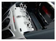
3. Remove the 4 screws of the OEM head unit
