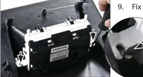
Fix OEM display with 2 screws
